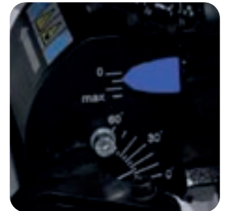
Continuous angle adjustment from 0 to 60 degrees.
