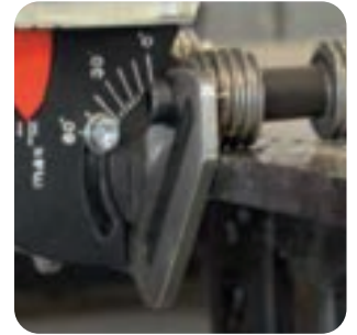
Continuous angle adjustment from 0 to 60 degrees.
